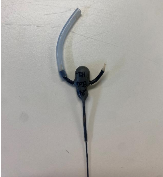
Figure 2. Transmitter of the brand Holohil BD-2 (weight 1.8 g), attached to a waist belt produced out of silicone tubing, PVC tubing and catgut (weight 0.5 g), designed after Burow et al. (2012).
