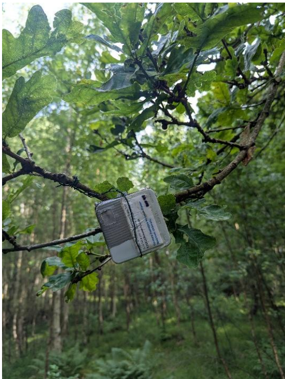
Figure 2. Acoustic recording device used in the inventory. AudioMoth recorders were placed inside protective cases and mounted on natural landscape elements.
